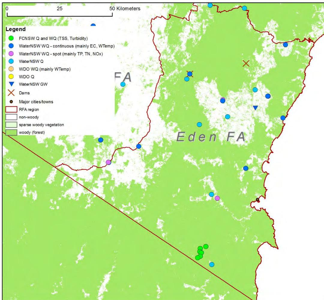
Figure A4. Water quality and quantity monitoring network the Eden FA. For water quality, only sites with 10 years of quarterly data are shown; for streamflow, only sites with 35 years of continuous data are shown.
