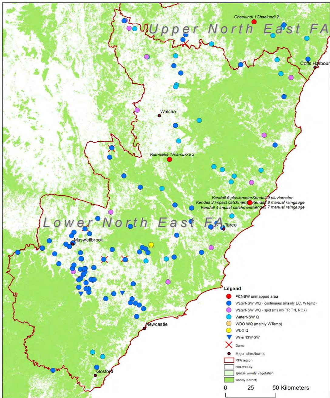
Figure A2. Water quality and quantity monitoring network the Lower North East FA. For water quality, only sites with 10 years of quarterly data are shown; for streamflow, only sites with 35 years of continuous data are shown. The approximate locations of the unmapped FCNSW sites are also shown – identifying the accurate locations of these sites are in progress.
