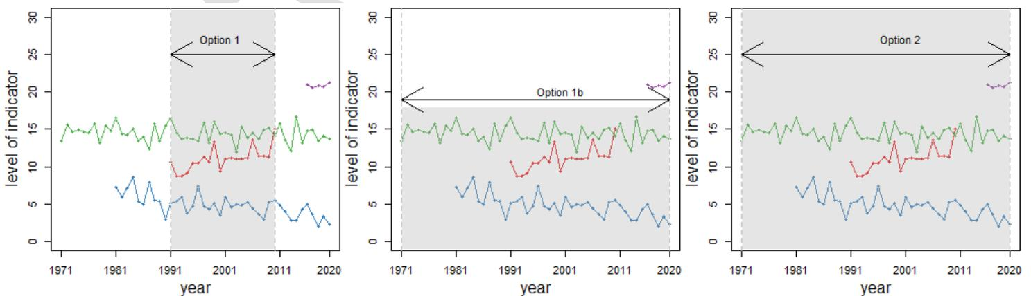
Figure 7. Comparison of the three alternative options for the temporal period of trend analysis (shaded). Hypothetical data from four individual monitoring sites are shown for illustration in different colours.
